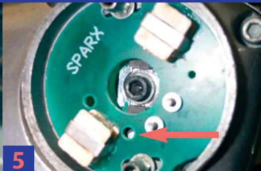
5 IF THE CAMSHAFT TURNS CLOCKWISE TURN THE ROTOR UNTIL YOU SEE SCREW IN THE BOTTOM HOLE THEN TIGHTEN THE ALLEN BOLT. THIS WILL GIVE YOU A GOOD STATIC TIME TO STROBE LATER.
