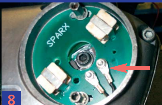
8 ROUTE THE STATOR PLATE WIRES VIA THE SHORTEST ROUTE (AVOIDING AC WIRES FROM THE ALTERNATOR AS THIS CAN CAUSE INTERFERENCE) TO THE ENGINE AND CUT TO LENGTH. USE OUTER SHIELDING AS SUPPLIED AND CRIMP TO THE TERMINAL CONNECTORS (CONNECT BLACK & WHITE WIRE TO RIGHT HAND TERMINAL).
