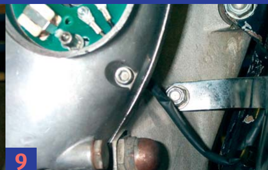
9 WHEN ROUTING THE STATOR PLATE WIRE TO THE ENGINE LEAVE A LITTLE J SHAPED LOOP IN THE WIRE CLOSE TO THE ENGINE AND LOOSELY CABLE TIE TO THE FRAME, THIS WILL STOP THE WIRE BREAKING DOWN UNDER VIBRATION ESPECIALLY ON NORTON ISOLASTIC FRAMED MODELS.
